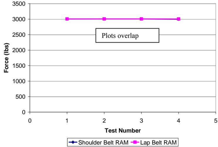
**Figure A 2.** Mean force values for the D-ring for all four tests
