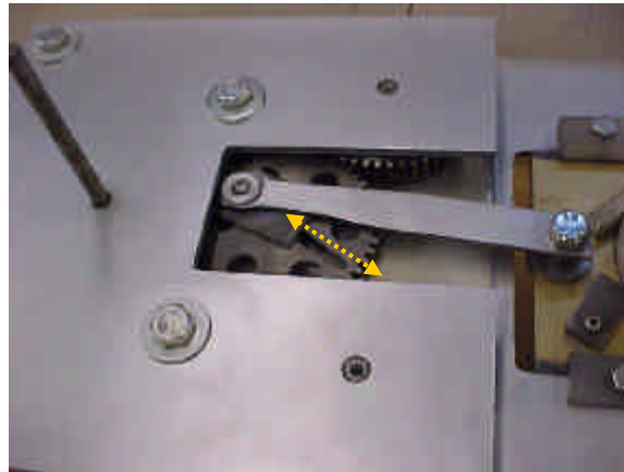
Figure 2: Photographic View of the Amplitude Adjustment Feature on the Testing Platform.
