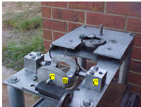
Figure. 10: Snapback Excitation Configuration of Testing Platform.
