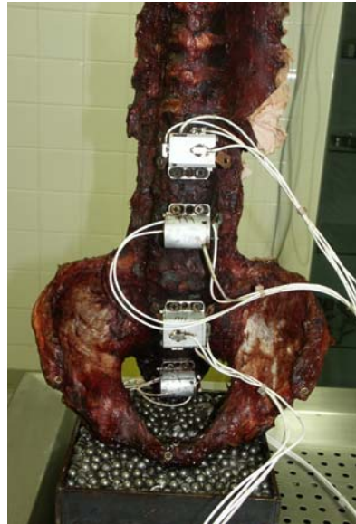
Figure 14: Checking of the alignment of the sensors boxes.
