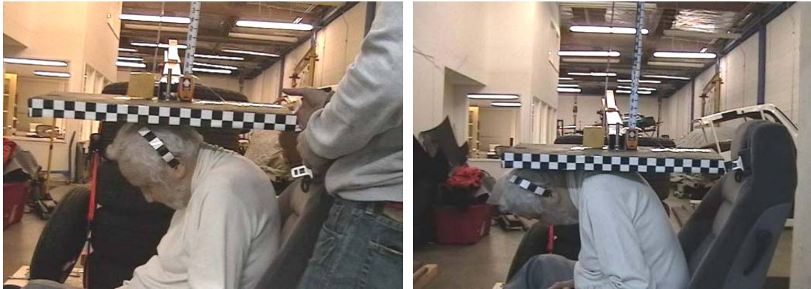
Figure 2: Platen Drop Test Setup, Human Volunteer Test Subject.
