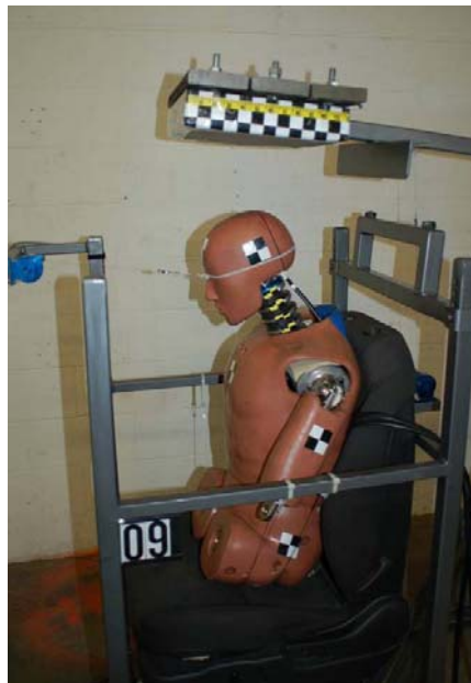
Figure 4: Pendulum Test Setup.
