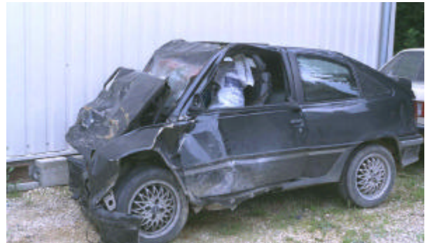
Figure 15. Damage to the Kadett E Model year '88 (1,998 ccm, 112 hp) after rescue of driver and passenger (EES = 65 kph, VDI5 = 5)
