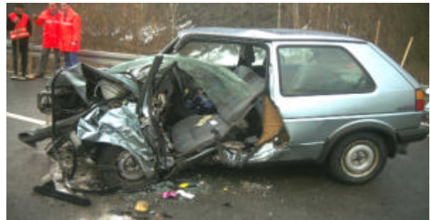
Figure 12. Damage to the Golf II Model year '87 (1,760 ccm, 90 hp) after rescue of driver (EES = 52 kph, VDI5 = 4)
