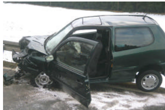
Figure 13. Damage to the Polo III Model year '96 (1,390 ccm, 60 hp) after rescue of driver (EES = 55 kph, VDI5 = 3)
