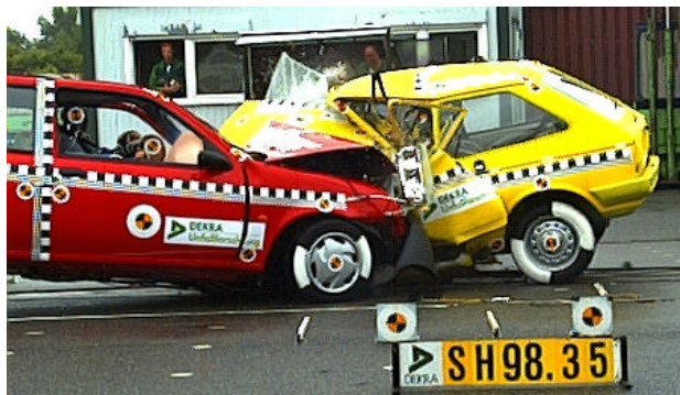
Figure 7. Car-to-car crash test Ford Fiesta model '98 (1,388 ccm, 90 hp) versus Ford Fiesta model '85 (1,117 ccm, 50 hp) both at 55 kph, 50 % frontal overlap
