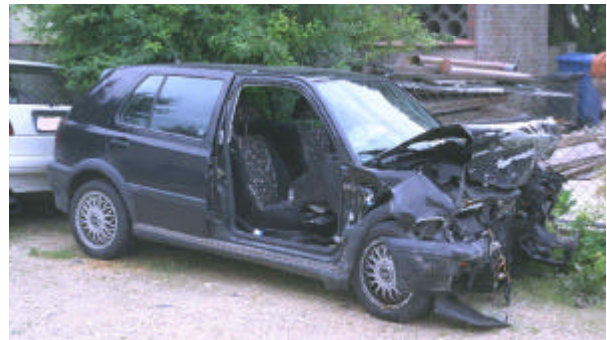
Figure 16. Damage to the Golf III Model year '94 (2,798 ccm, 165 hp) after rescue of driver (EES = 55 kph, VDI5 = 4)
