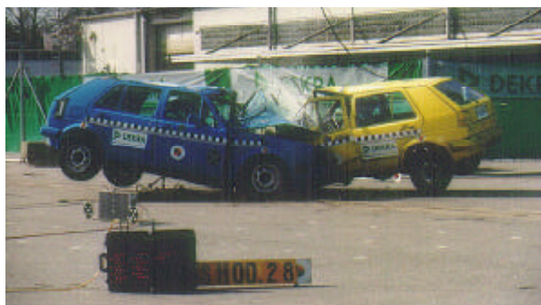
Figure 24. Car-to-car crash test VW Golf II model year '87 (1,570 ccm, 75 hp) versus VW Golf II model year '87 (1570 ccm, 75 hp) both at 55 kph, 50 % frontal overlap
