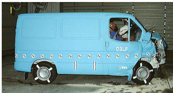
Figure 4. Deformation of the non car derived van showing reasonably stable passenger cell.
