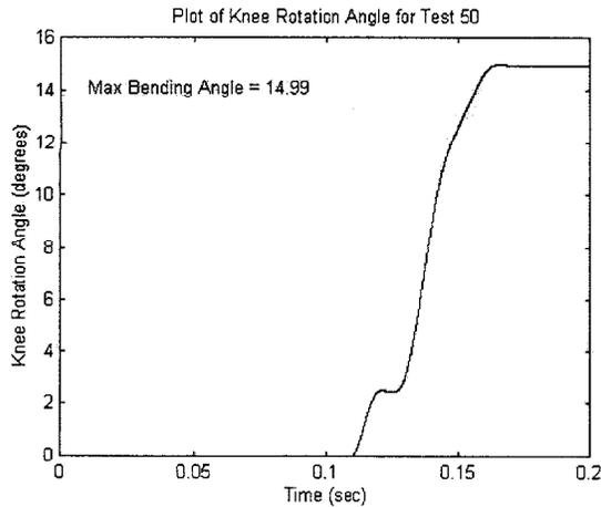
Figure 7. Sample output for knee rotation angle.
