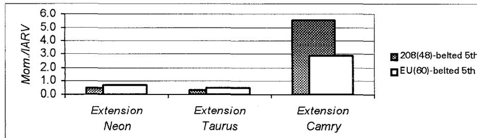
**Figure 14. Right front passenger neck bending moment comparison of the 5<sup>th</sup> percentile female Hybrid III between the two test types.**
