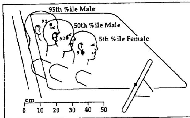
**Figure A1. Relative driver dummy sitting position**
