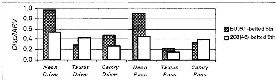
Figure 4. Chest displacement comparison
