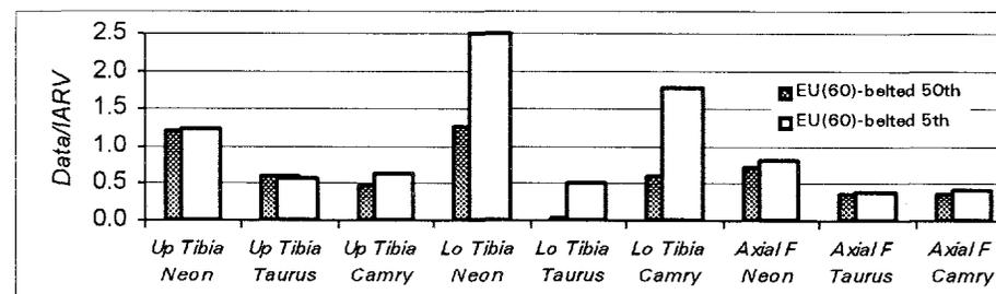
Figure 10. Driver right leg tibia comparison between the two dummy types in the EU-offset test.
