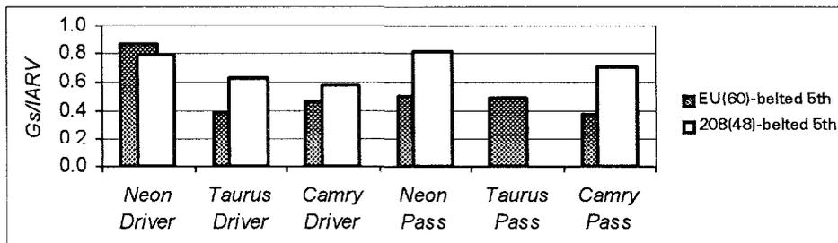
Figure 3. Chest acceleration (3ms clip) comparison
