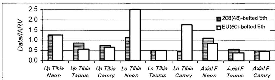
Figure 8. Driver right leg tibia comparison of the 5th percentile female dummy between the EU-offset and the FMVSS No. 208 tests.
