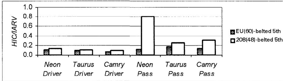
Figure 2. Head Injury Criterion (HIC) comparison.
