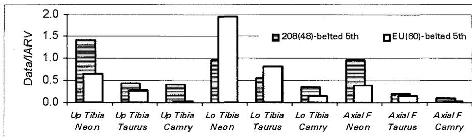
Figure 7. Driver left leg tibia comparison of the 5th percentile female dummy between the EU-offset and the FMVSS No. 208 tests.
