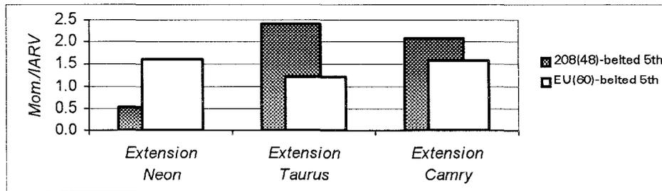
**Figure 13. Driver neck bending moment comparison of the 5<sup>th</sup> percentile female Hybrid III between the two test types.**
