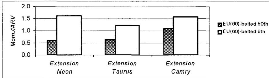
**Figure 11. Driver neck bending moment comparison between the two dummy types in EU-offset test.**
