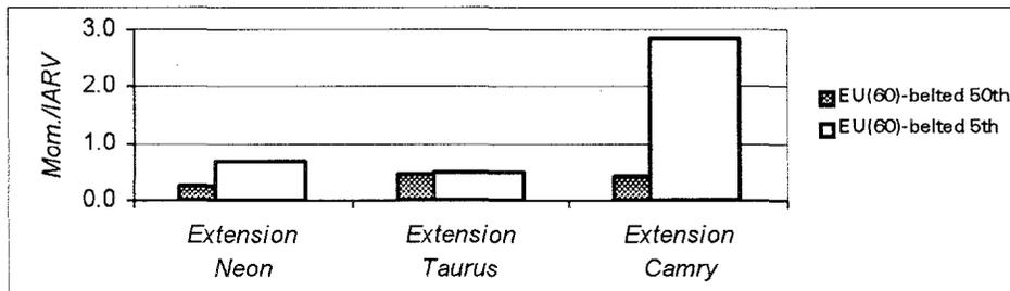
**Figure 12. Passenger neck bending moment comparison between the two dummy types in EU-offset test.**
