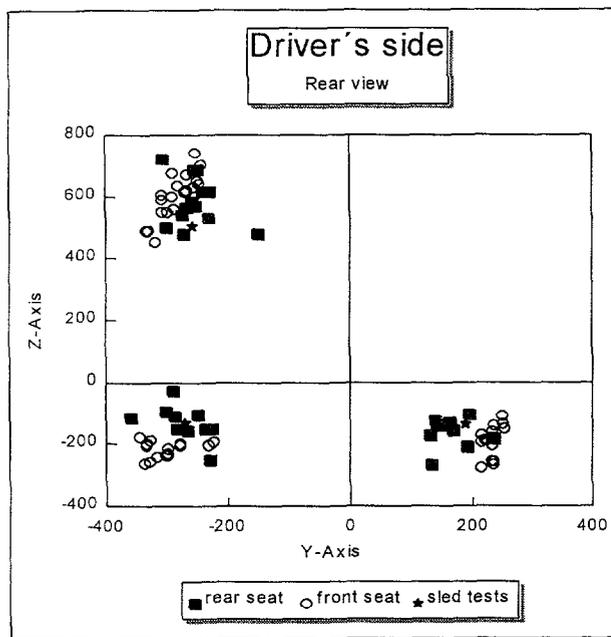
**Figure 1:** Position of the belt-anchoring points of various cars, measuring from the H-point of the dummy, in the direction of traffic. Also shown are the anchoring points as they are used in the testing in Section 7.
