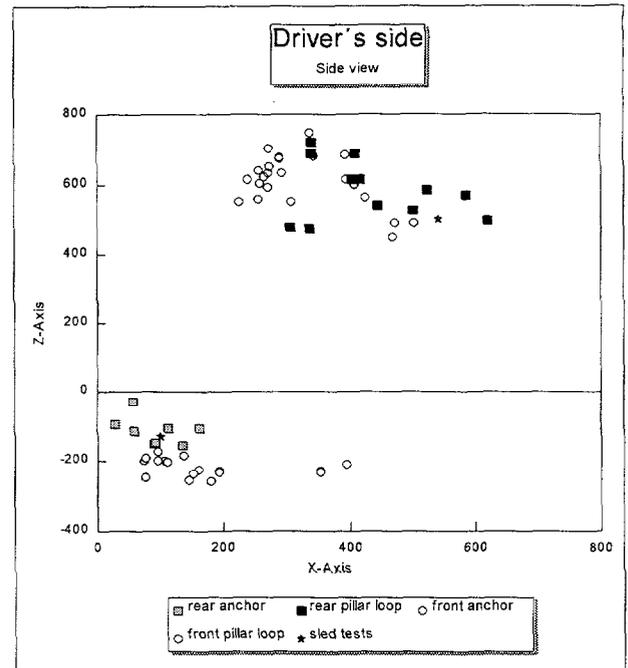
**Figure 2:** Position of the belt-anchoring points of various cars, measuring from the H-point of the dummy, in the direction of traffic. Also shown are the anchoring points as they are used in the testing in Section 7.
