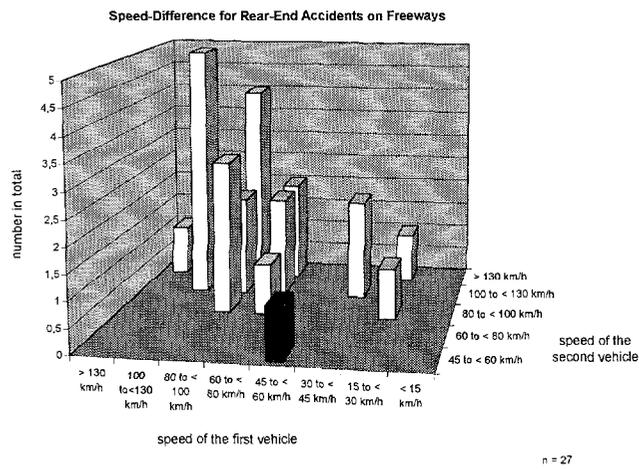
**Figure 9. Driving speed differences of passenger cars involved in rear-end accidents on highways and autobahns /4/**
