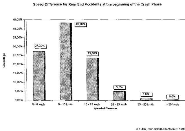
**Figure 10. Speed difference at the beginning of the crash phase for rear-end accidents of two passenger cars /5/**
