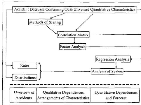
**Figure 12. Scheme of accident data analysis**
