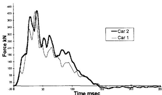
Figure 6.- Interface force calculated in car to car offset impact.
