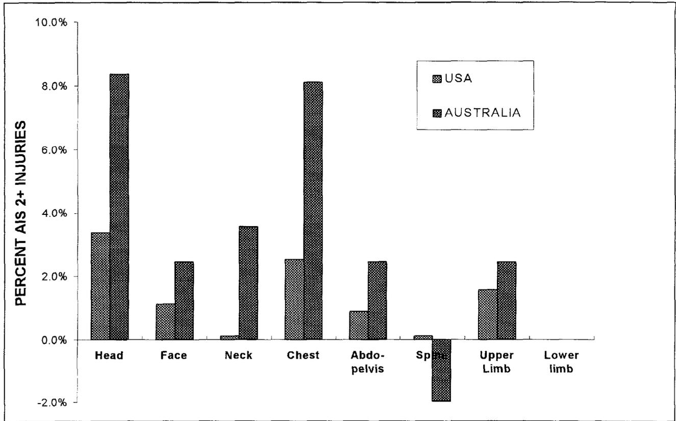
*Figure 2; Difference in percent of injuries for drivers with the adjusted seat belt only and the original seat belt and airbag restraints.*
