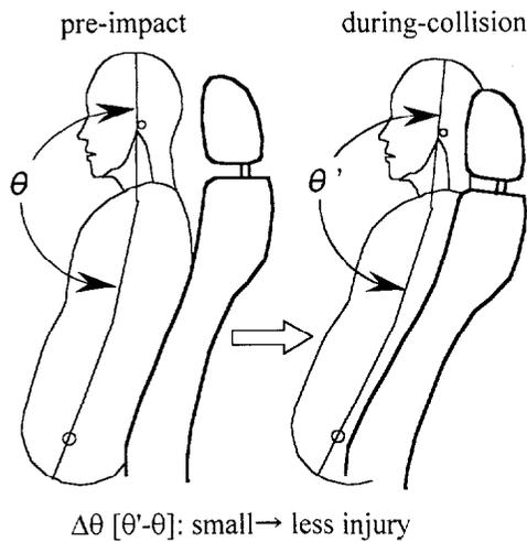
**Figure 1. Desirable occupant motion during impact in low-speed rear end collision.**
