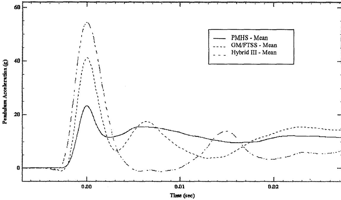
Figure 26 - Pendulum Acceleration at 4 m/sec, Inversion Impacts
