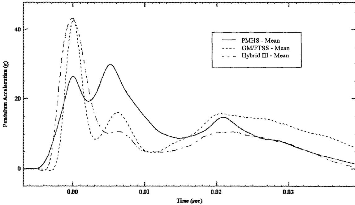
Figure 27 - Pendulum Acceleration at 4 m/sec, Eversion Impacts
