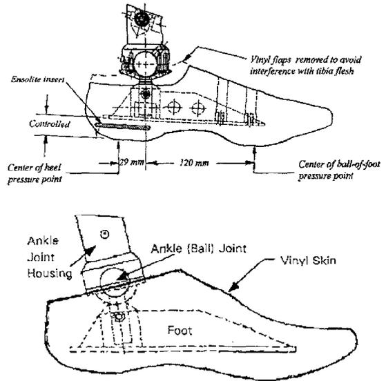
Figure 1 - The Hybrid III Foot Assembly
