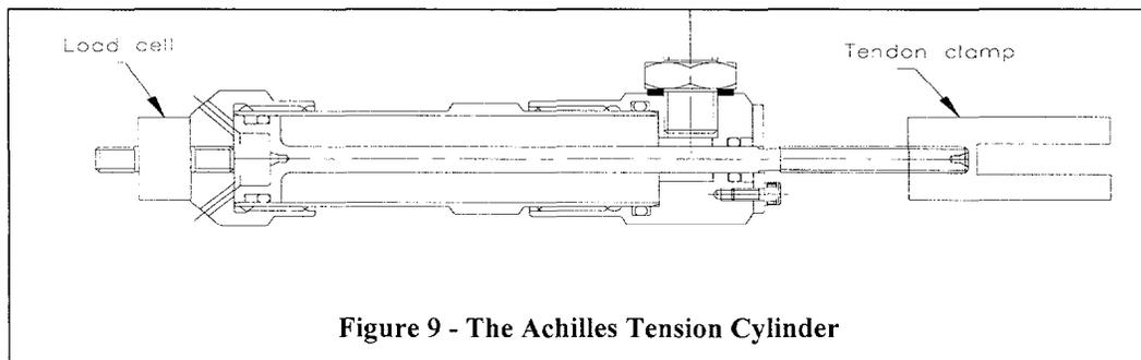
Figure 9 - The Achilles Tension Cylinder
