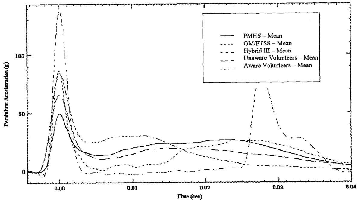
Figure 19 - Pendulum Acceleration at 6m/sec - Toe Impacts
