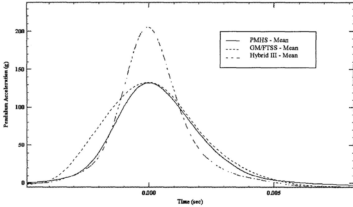
Figure 24 – Tibial Pendulum Acceleration at 4 m/sec, Heel Impacts
