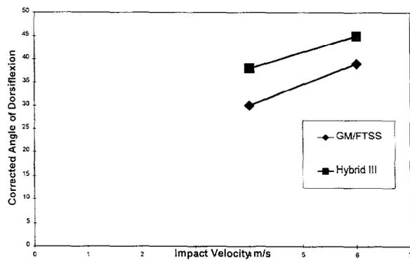
Figure 16 - Dummy Toe Impacts Dummies
