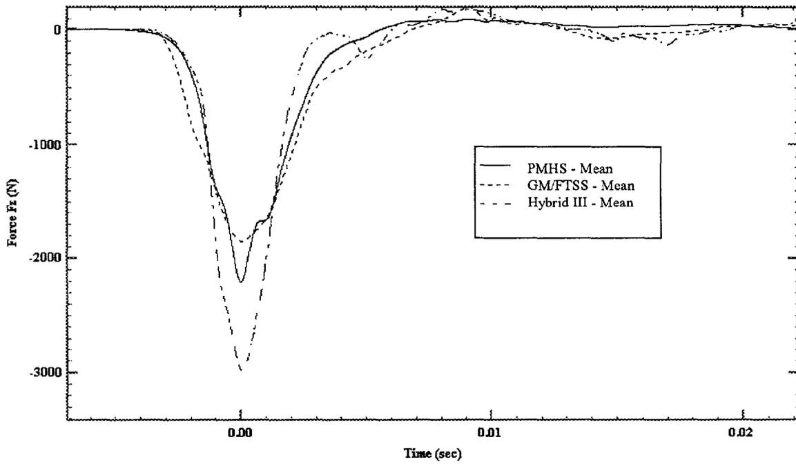
Figure 25 – Tibial Force  $F_z$  at 4 m/sec, Heel Impacts
