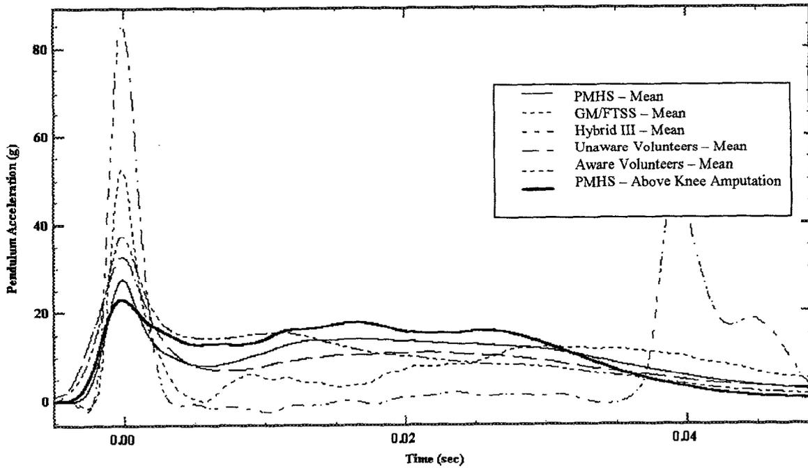
Figure 18 - Pendulum Acceleration at 4m/sec - Toe Impacts
