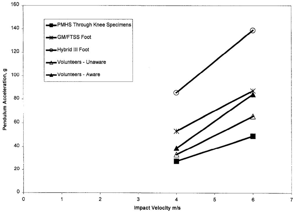
Figure 32 – Mean Peak Responses for Toe Impacts – Pendulum Acceleration
