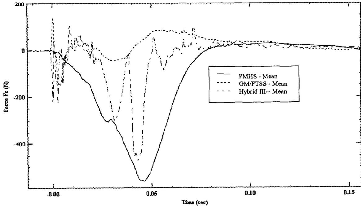
Figure 20 – Tibial Force Fz at 4m/sec - Toe Impacts
