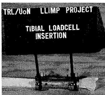
Figure A1 - Cutting Jig In-Situ on Tibia
