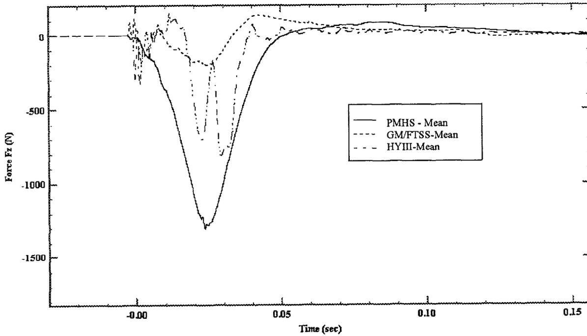
Figure 21 – Tibial Force Fz at 6 m/sec - Toe Impacts
