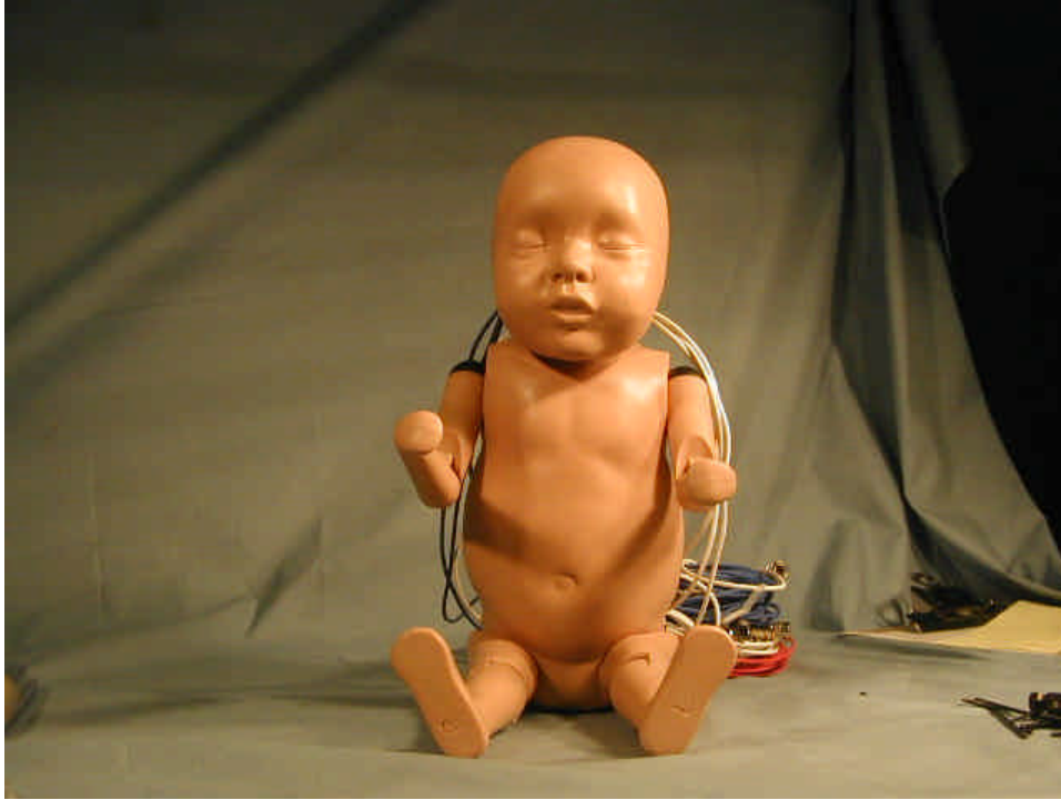
Figure 1: Aprica 2.5 Kg Infant Test Dummy With Instrumentation.
