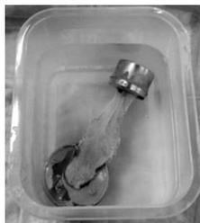
Figure 4: MCL specimen potted at both bone ends kept in saline solution
