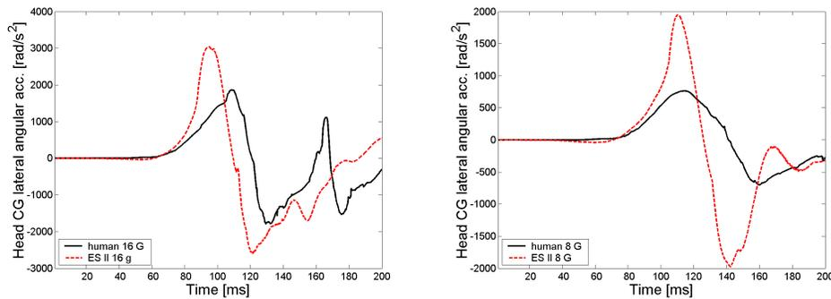
Figure 10: Head CG lateral angular acceleration. Human model compared with dummy model.
