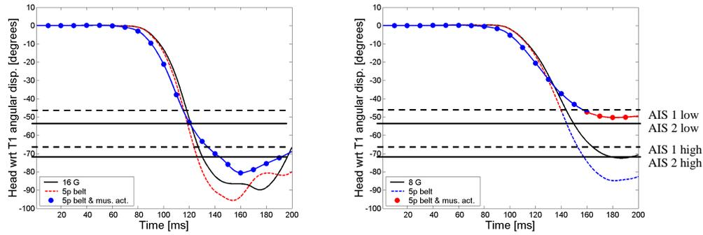
Figure 7: Head wrt. T1 lateral angular displacement. Human model situation without belts compared with 5-point belt and with 5-point belt plus 50% neck muscle activity.
