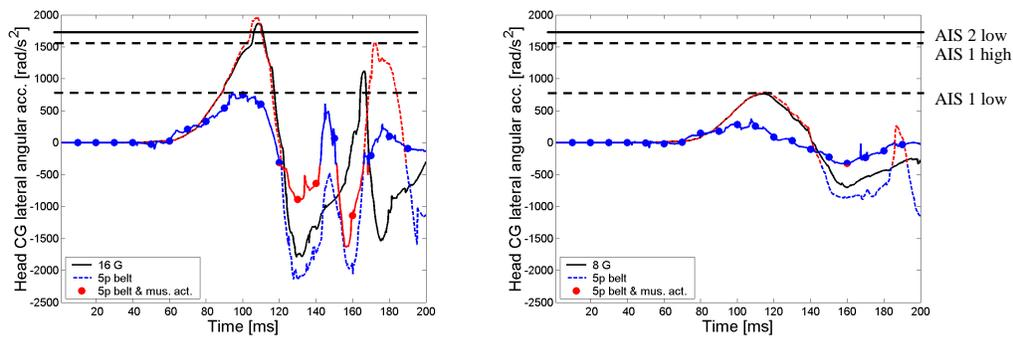
Figure 8: Head lateral angular acceleration. Human model situation without belts compared with 5-point belt and with 5-point belt plus 50% neck muscle activity.
