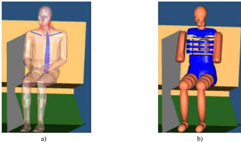
Figure 2: a) Human model in side facing seat; b) Dummy model in side facing seat.
