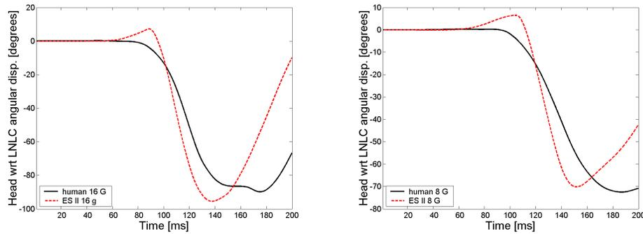
Figure 9: Head w.r.t. LNLc (lower neck load cell) or w.r.t. T1 lateral angular displacement. Human model compared with dummy model.
