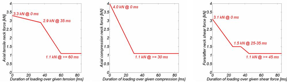
Figure 5: Tolerance levels for tension, compression and shear for frontal neck loading criteria FNIC proposed by EEVC Working Group 11 (Lowne, 1996).
