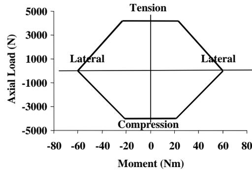
Figure 6: Tolerance levels for neck lateral load  $N_{ij}$  criteria proposed by Soltis (2001).
