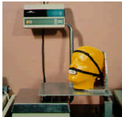
Figure 4: Manikin head within the support box being measured for CG_x
