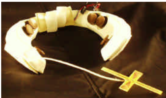
Figure 1: Six accelerometers, FM-antenna, and rechargeable battery pack.
