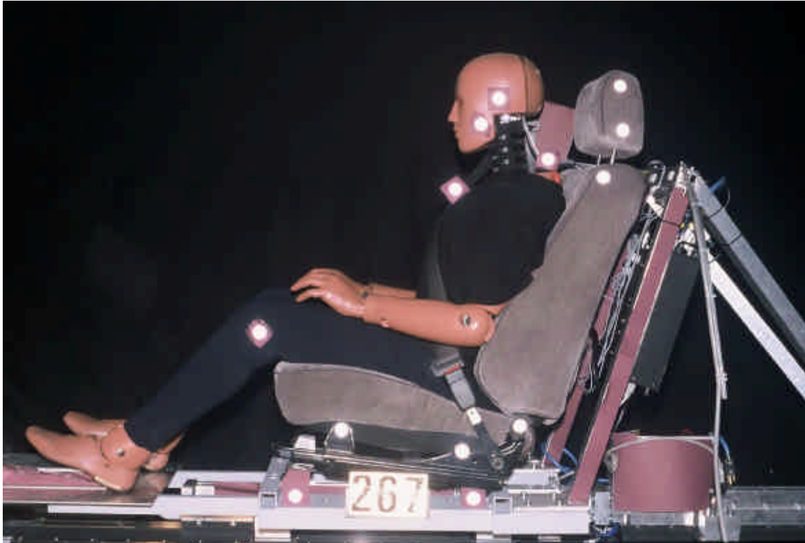
Figure 1: Lateral view of the dummy on the sled with the seat fully rearward and thus the outboard seat belt anchor points (not visible) in the forward condition. The inboard lap anchor (visible) moves with the seat.
