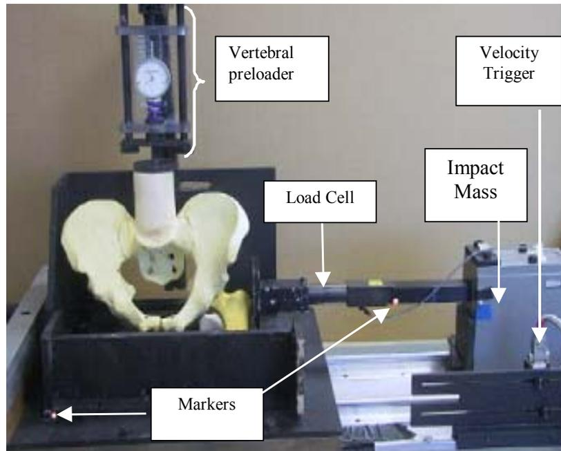
Figure 4: Pneumatic impact test set-up. Each pelvis (plastic model shown) was seated and constrained as shown, including compressive pre-load and a contralateral rigid plate. The impact mass struck the greater trochanter. Impact force was measured with the load cell, while pelvic compression was obtained from high-speed films of marker motion.
