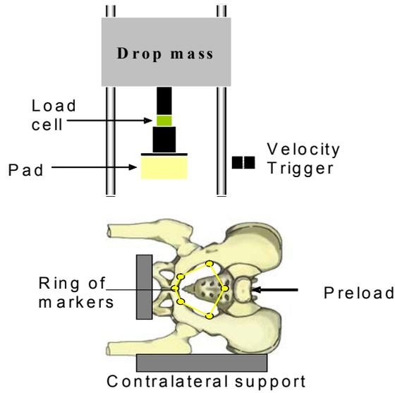
Figure 2: Schematic of drop tower impacts. Isolated bone-ligament specimens were positioned on their side with femurs flexed at approximately 90 degrees, potted contralaterally in PMMA, compressively preloaded through the spine and supported with frictional restraint at the ischial tuberosities.
