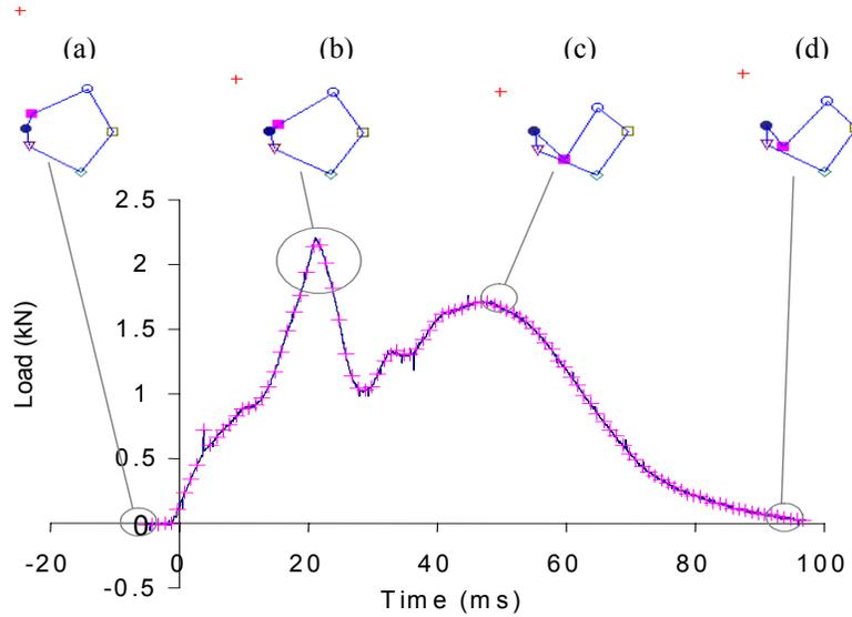
Figure 5: Force-time plot with corresponding camera images (above) for the padded impact of pelvis #76. (a) Velocity trigger initiates data capture prior to impact, (b) fracture of right superior pubic ramus at 25.75 ms, (c) maximum impactor displacement at 44.75 ms, (d) rebounding impactor loses contact with pelvis at 96.75 ms. The single marker on the falling impactor is shown as a cross.
