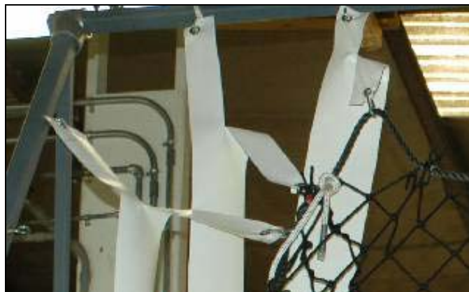
Figure 19: Energy absorbing strips attached to catcher frame and net.
