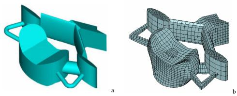
Figure 2: Parametrically defined (a) solid model of the cervical vertebra and (b) mesh.
