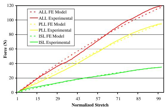
Figure 6: Ligament finite element (FE) models compared to the quasi-static experimental data for the ALL, PLL, and ISL.
