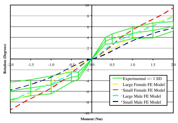
Figure 13: Finite element (FE) models compared to the experimental data for the C5-C6 motion segment rotational response in axial rotation.
