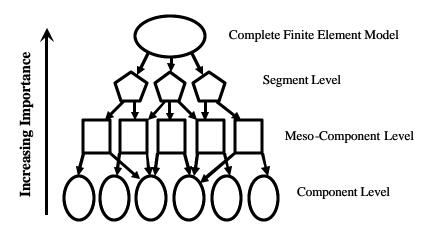
Figure 1: Verification and validation hierarchy.
