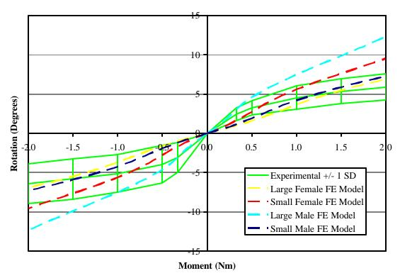
Figure 12: Finite element (FE) models compared to the experimental data for the C5-C6 motion segment rotational response in lateral bending.
