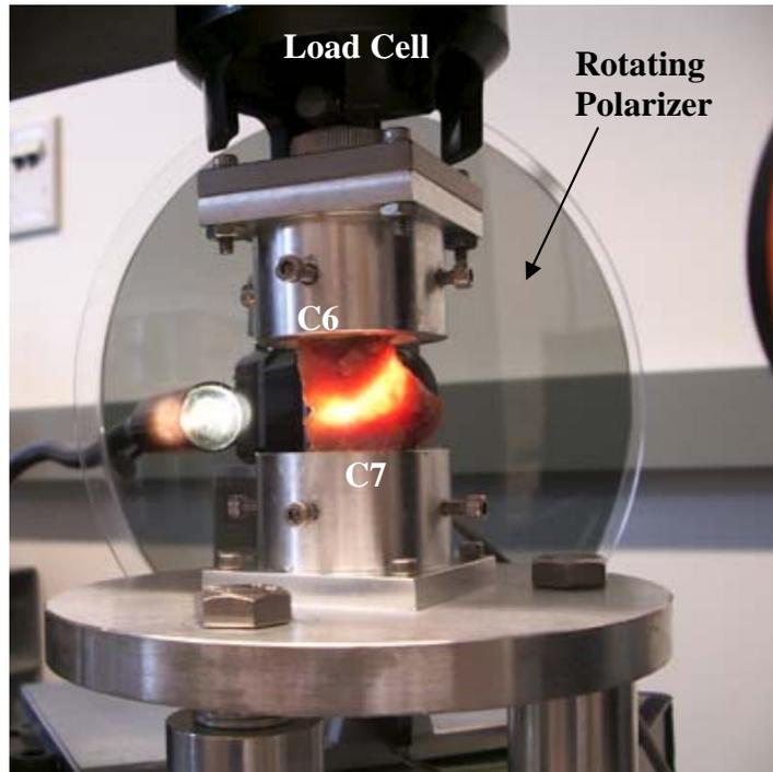
Figure 1: Right C6/C7 facet joint mounted to Instron with joint space illuminated by focused light source. Behind the specimen and test device is the rotating polarizer and focused light source.
