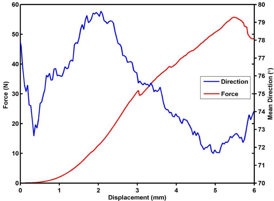
Figure 4: Force and mean alignment direction during distraction for specimen #C893-C67L. Direction is measured with respect to the positive X-axis, so the direction of loading was 90° (along Y-axis).
