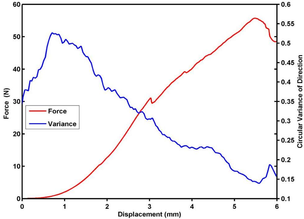
Figure 5: Force and directional variance during distraction for specimen #C893-C67L. The decrease in variance with increasing displacement indicates increasing alignment in the X- and Y- directions.
