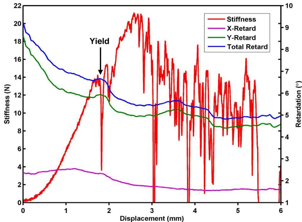
Figure 7: Stiffness and mean retardation during distraction for specimen #C893-C67L. X- and Y-components of mean retardation (magenta & green, respectively) are shown, as well as total mean retardation (blue). The ligament yield point is indicated by an arrow; yield may correspond with changes in retardation.
