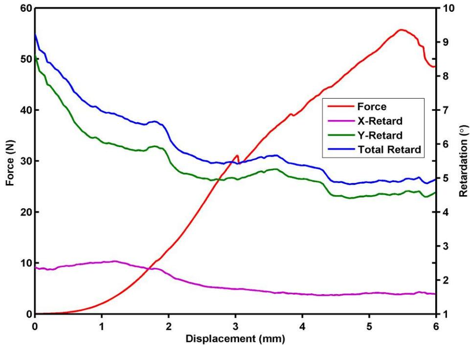
Figure 6: Force and mean retardation during distraction for specimen #C893-C67L. The X and Y components of mean retardation (magenta & green, respectively) are shown, as well as mean total retardation (blue). The decrease in retardation with increasing distraction indicates the decreasing mean alignment through the thickness of the ligament (Z-direction).
