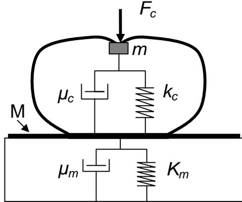
Figure 1: Mechanical model of chest atop compliant bed/stretchers.
