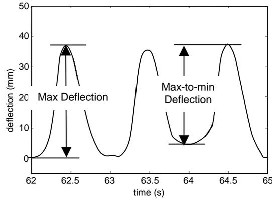
Figure 2: Methods of calculating maximum deflection, and estimated and measured deflection. Max deflection is simply the magnitude of deflection. Max-to-min deflection is calculated as the maximum of each wave minus the previous minimum.
