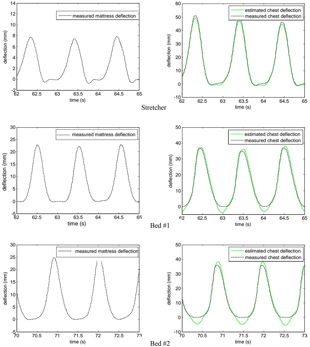
Figure 3: Exemplar deflection time-histories for the mattress and manikin chest. Manikin chest deflections (right panels) are shown with estimated deflections overlaid with measured deflections. Zero deflection indicates the resting position of the chest or mattress in the absence of any applied CPR force. Positive deflection values indicate mattress or chest compression.
