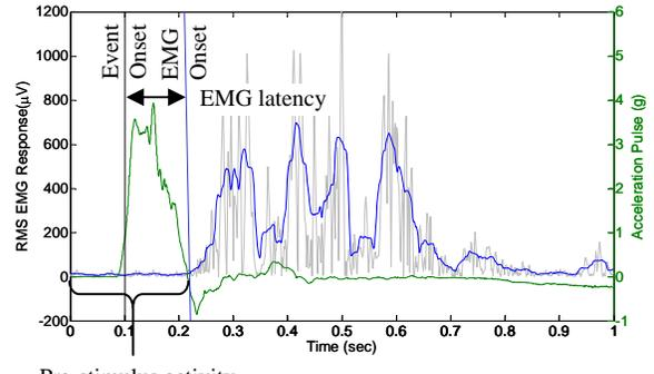
Figure 7: Sled acceleration superimposed over raw EMG data and smoothed 25 ms RMS data for a single human volunteer.
