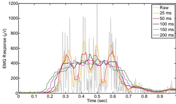
Figure 6: Raw EMG and Root mean squared (RMS) plots using 25, 50, 100, 150 and 200 ms smoothing windows for the right SCM muscle for a subject.
