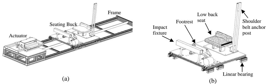
Figure 1: (a) Schematic of the low-speed acceleration seating buck (LASB) (b) Schematic of the seating buck assembly.
