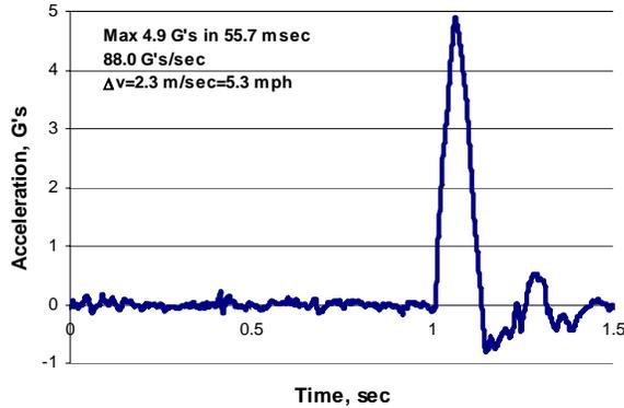
Figure 2: Bumper car to wall acceleration pulse.
