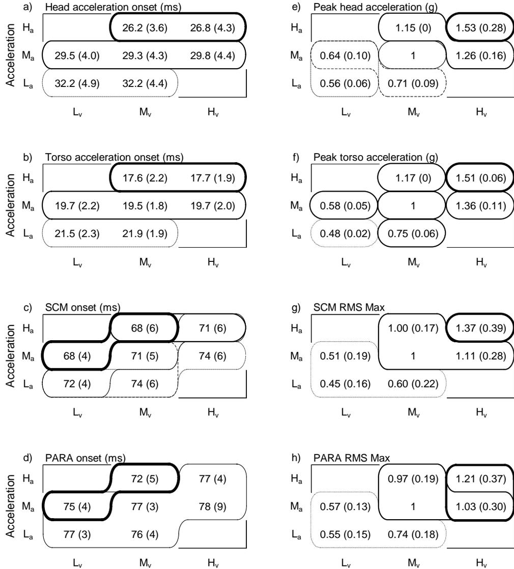
Figure 4: Mean and standard deviation of times for the (a) head acceleration onset, (b) torso acceleration onset, (c) SCM onset latency and (d) PARA onset latency; and normalized peak amplitudes for (e) head acceleration, (f) torso acceleration, (g) RMS SCM activity and (h) RMS PARA activity as a function of perturbation acceleration and velocity. The borders encircle homogeneous groups of data and increasing line weight corresponds to earlier times and increasing amplitude.
