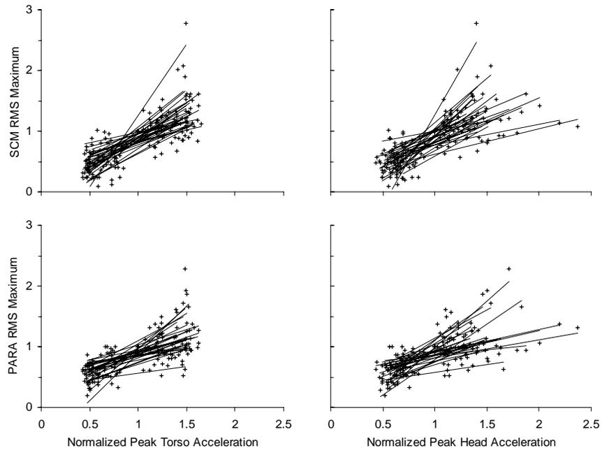
Figure 6: Linear regression analyses demonstrating the presence of a correlation between the amplitude of the neck muscle EMG (SCM, top row; PARA, bottom row) and the amplitude of both the torso (left column) and the head (right column) accelerations. Each straight line represents the least-squares best fit line through an individual subject's data.
