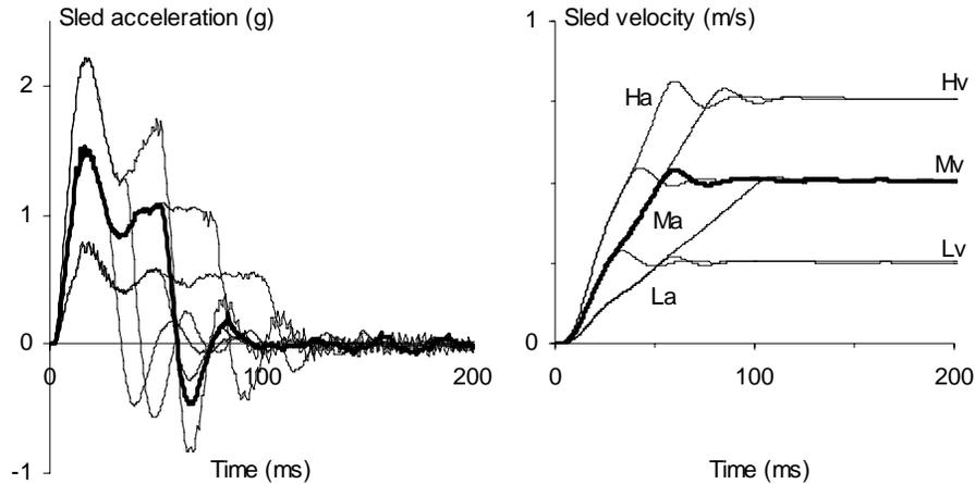
Figure 2: Acceleration and velocity of the seven perturbations. Superimposed acceleration vs. time traces (a) and velocity vs. time traces (b) show similarities between the perturbations. The bold lines depict the standard perturbation (MaMv) in both upper panels. Sled acceleration: low La, medium Ma, and high Ha; and sled velocity: low Lv, medium Mv, and high Hv.
