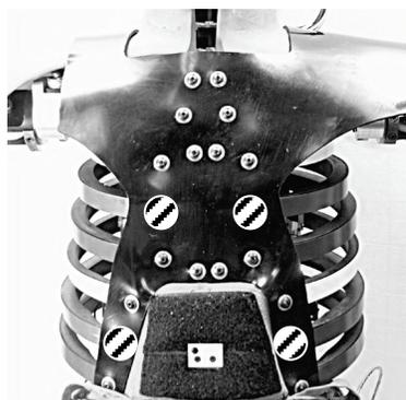
Figure 2: Anterior view of the THOR ATD thorax structure with the locations of the multi-dimensional deflection sensor shown in hatched circles at the left and right aspect of the fourth and the eighth ribs.
