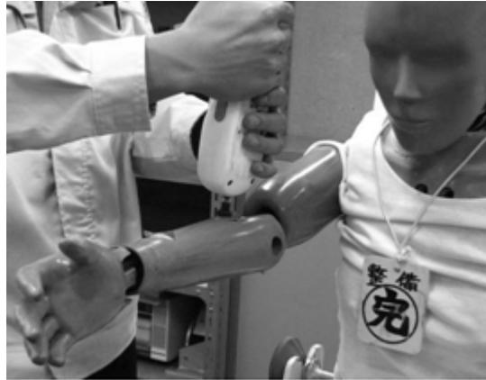
Figure 6: Measurement of joint stiffness
