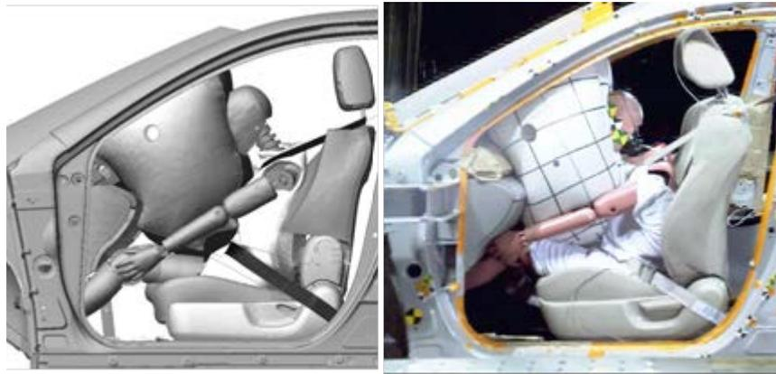
Figure 18: Comparison of Sled Test Kinematics (70 ms)
