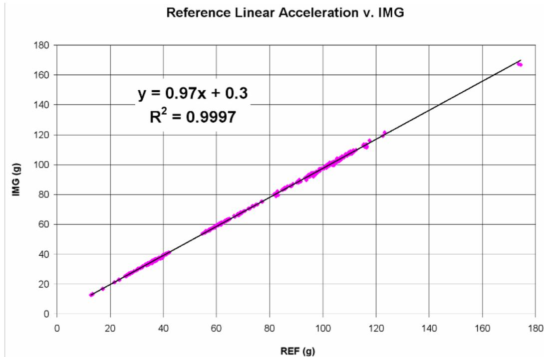
Figure 2: Peak Reference Linear Acceleration vs. Peak IMG PCB Linear Acceleration (n=439 tests).
