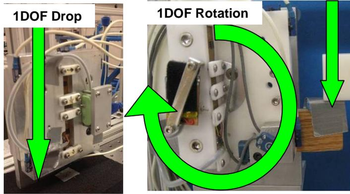
Figure 1: Aluminum Drop Testing Fixture Used in the Current Study.
