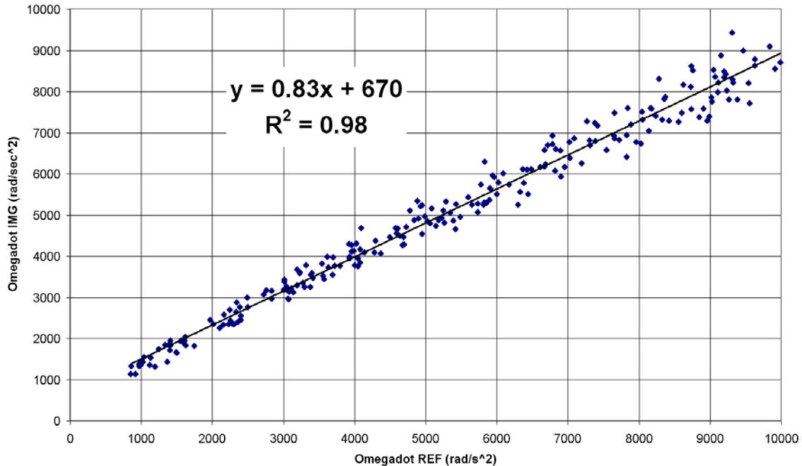
Figure 3: Peak Reference Angular Acceleration vs. Peak IMG PCB Angular Acceleration (n=235 tests).
