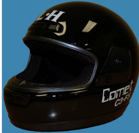
Figure 1: Helmet model (L'H Comet C3-FS) used in tests was certified to DOT and Snell M95 standards. The visors of the helmets were cut prior to testing to accommodate the ball arm of the monorail and trolley assembly.
