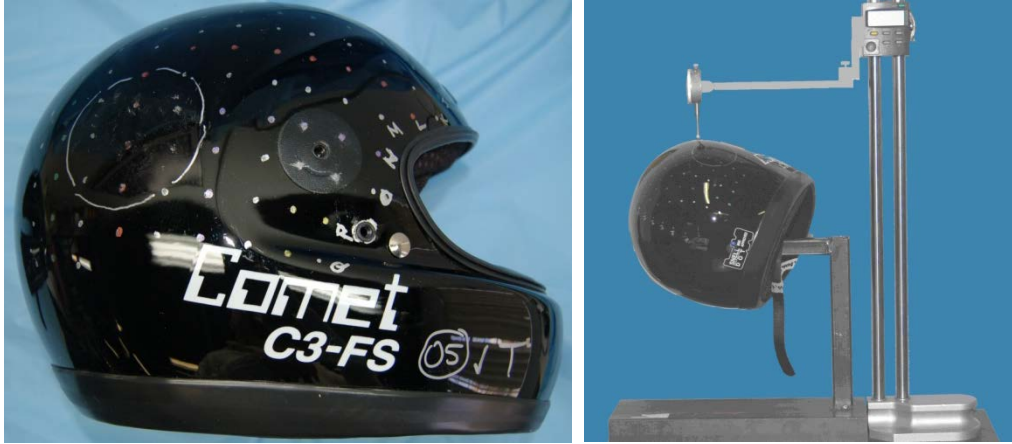
Figure 3: Left: General arrangement of grid and helmet thickness measurement locations. Right: Height gage apparatus used to measure helmet thickness over each grid location.
