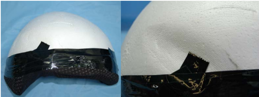
Figure 5: Views of exterior surface of energy absorbing liner following 180J test with curbstone anvil. Left: Overall view of impact side (helmet cut in half). Right: Close-up of the localized liner deformation due to penetration of the curbstone anvil into the shell and liner.
