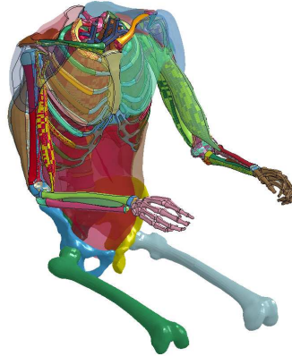
Figure 1: FE representation of the THOMO reference model. Combination of bone, flesh, muscle and internal organs structure.
