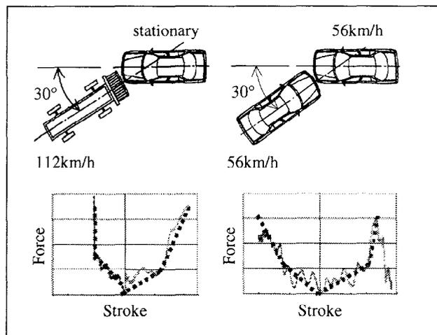
**Figure 13. Comparison of Force-Stroke characteristics**
