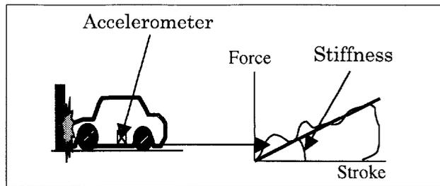
**Figure 10. Definition of vehicle stiffness**
