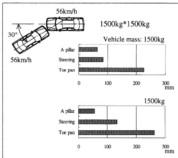
**Figure 11. Vehicle deformation (vehicle-to-vehicle)**
