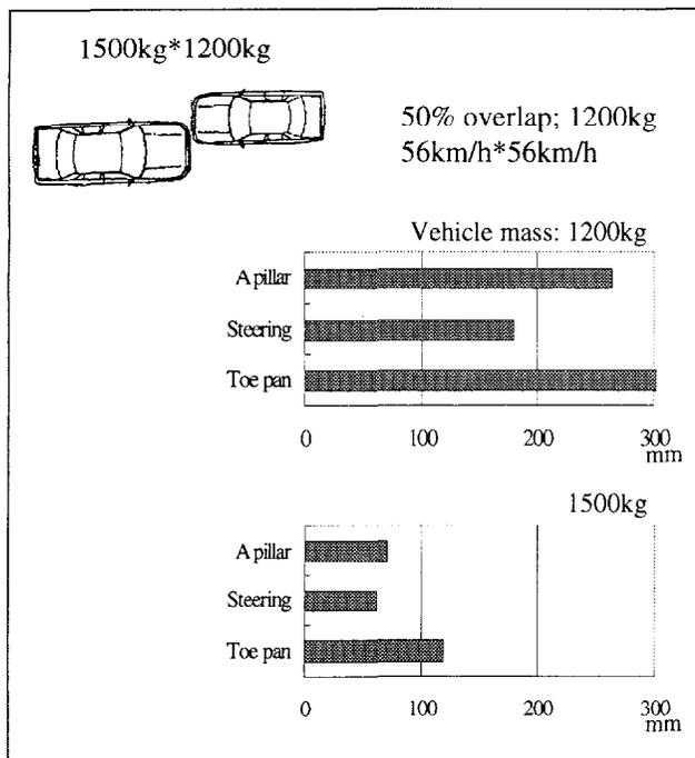
Figure 7. Vehicle deformation (vehicle-to-vehicle)
