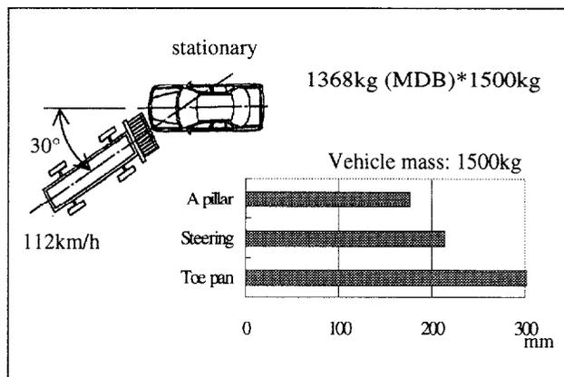
**Figure 12. Vehicle deformation (vehicle-to-vehicle)**
