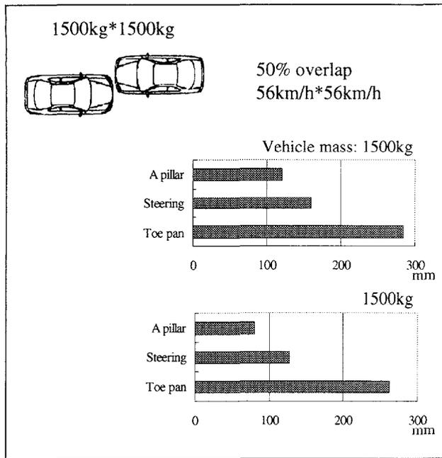
Figure 6. Vehicle deformation (vehicle-to-vehicle)
