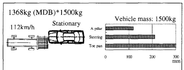
**Figure 15. Vehicle deformation (MDB-to-vehicle)**
