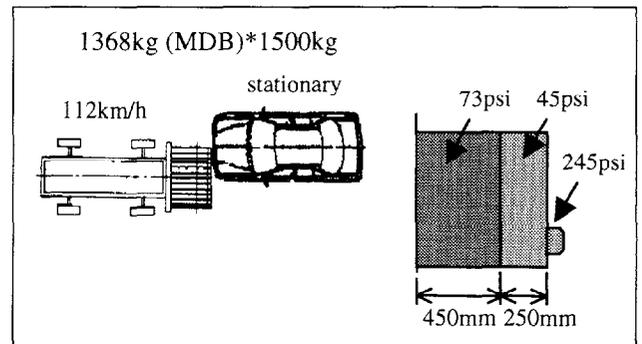
**Figure 14. Test method of MDB-to-vehicle**
