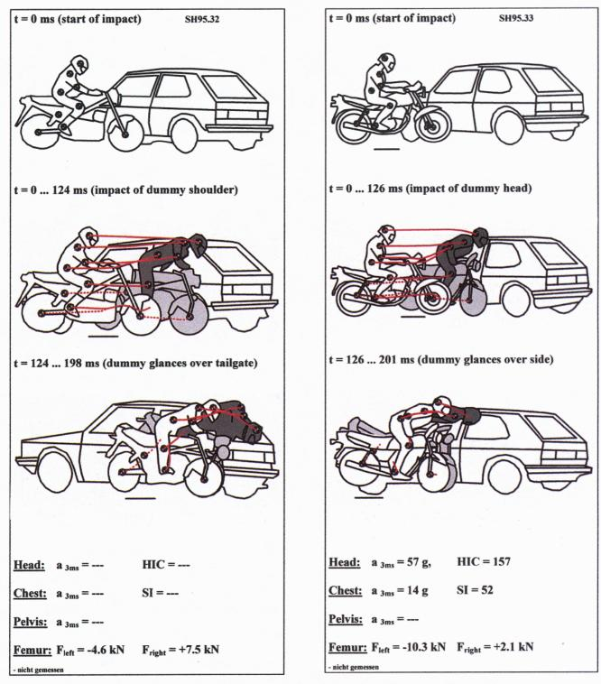
Figure 20. Results of film evaluations of a full-scale crash test between moving motorcycle and moving passenger car and measured femur loadings of the dummy (Configuration 414 in ISO/DIS 13232) Figure 21. Results of film evaluations of a full-scale crash test between moving motorcycle and stationary passenger car and measured head, chest and femur loadings of the dummy (Configuration 414 in ISO/DIS 13232)
