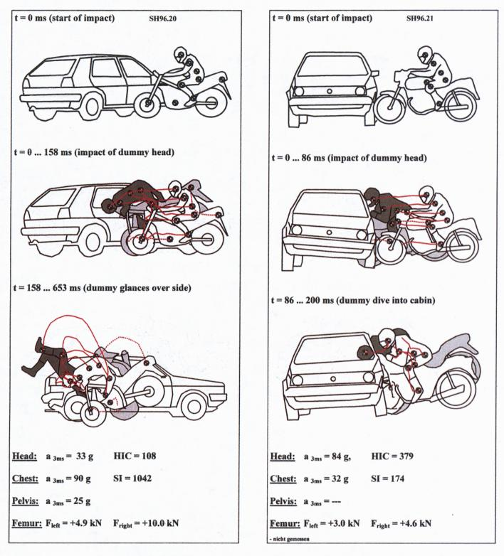
Figure 22. Results of film evaluation of a full-scale crash test between moving motorcycle and moving passenger car and measured loadings of the dummy (Configuration 414 in ISO/DIS 13232)
