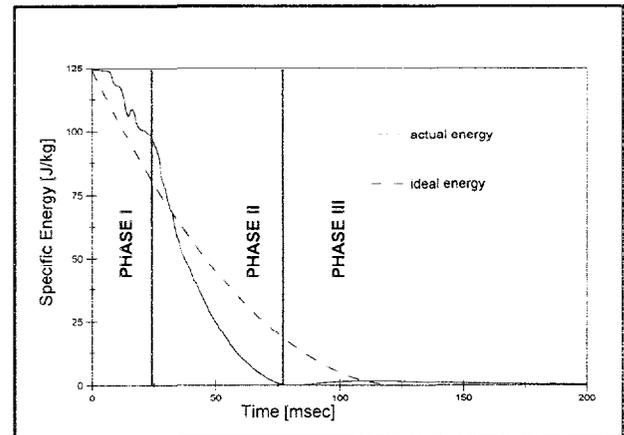
Figure 3. Division of the Typical Vehicle Specific Energy Curves into 3 distinct phases.
