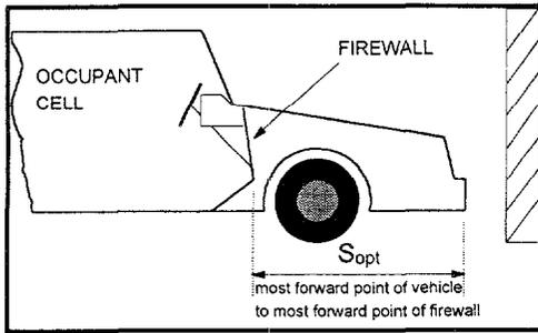
Figure 1. Optimum vehicle crush distance.
