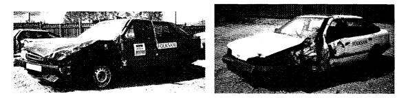
Fig. 9. The Saab 9000 and the Ford Scorpio in the crash test.
