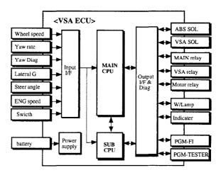
Figure 11. ECU block diagram
