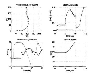
Figure 5. Simulation results (without front-brake control)
