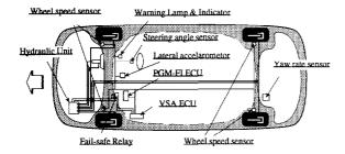
Figure 8. Construction of the VSA system.
