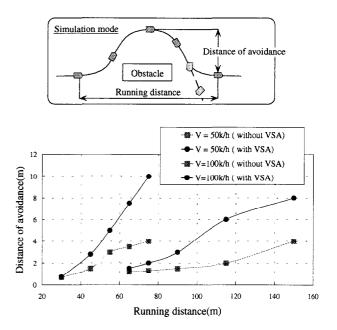
Figure 15. Capacity of crash avoidance. (simulation result)
