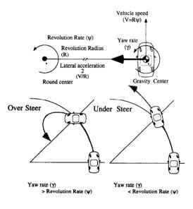
Figure 13. Yaw rate and revolution angular rate
