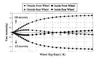
Figure 4. Effect of wheel braking on vehicle rotating
