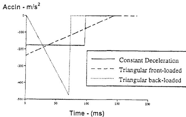
Figure 10. Comparison of simple shaped deceleration pulses for a ride down distance 0.8m.
