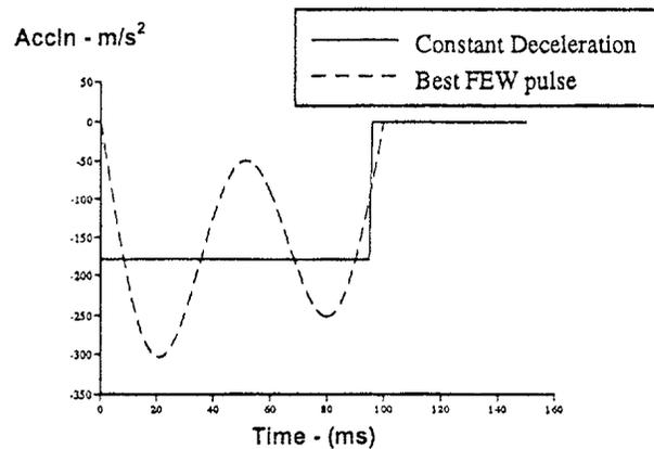
Figure 13. Comparison of doubled humped FEW and constant deceleration pulses.
