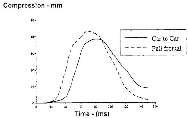
Figure 22. Comparison of chest compression for car to car and full frontal rigid wall impacts.
