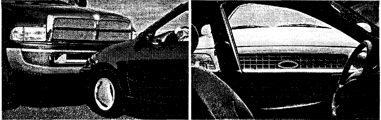
Fig. 3: Geometrical comparison between car and sports-utility vehicle. There are major discrepancies between the two front structures and between front and side. (Courtesy of IIHS (IIHS, 1998))
