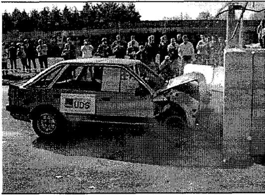
**Figure 5. Vehicle after 52km/h frontal crash.**
