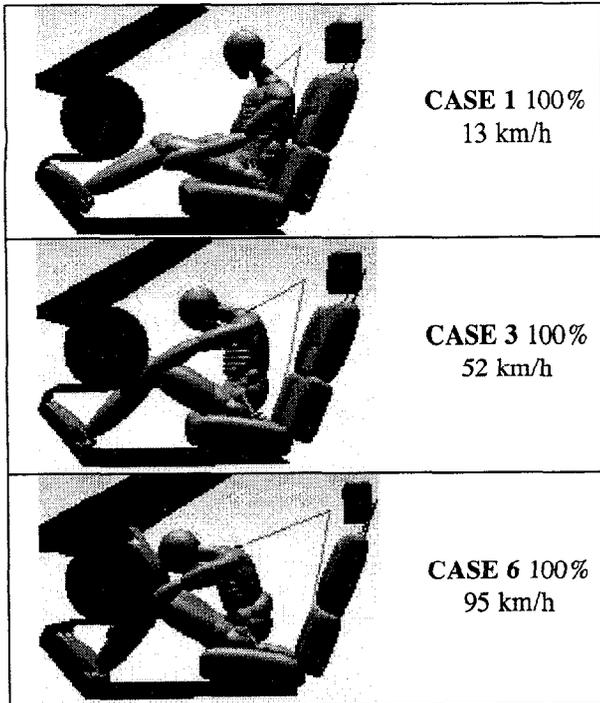
Figure 8. Simulation of maximum occupant movement without intrusions.
