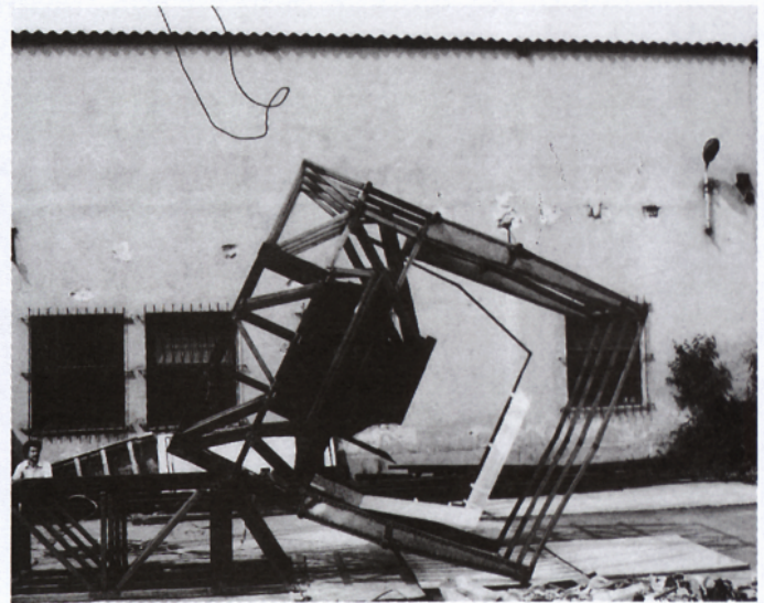
Fig. 6. Rollover test on a contracted multiple ring of IK 255 bus in 1985. This 2,5 m long, 8120 kg frame-segment contained 2 reinforced rollbars and 2 window-rings. (There was used a wood-surface.)
