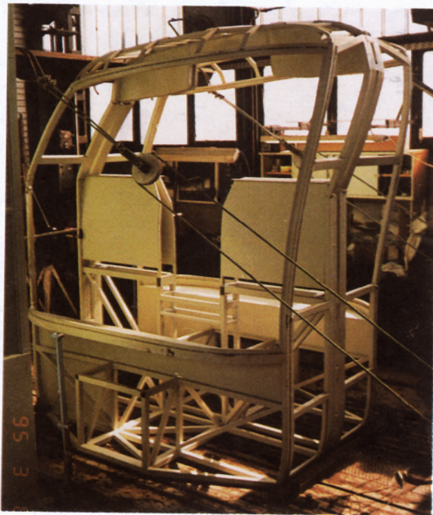
Fig. 9. Laboratory bending test for mathematical calculation of bus roof strength. Measuring the whole deformation process and the exact places of real plastic hinges the rollover simulation can be easily carried out with a simple iteration.
