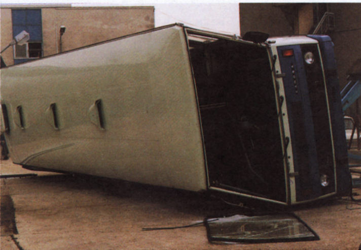
Fig. 5. Usual deformation shape of the superstructure after rollover test from 800 mm height.
