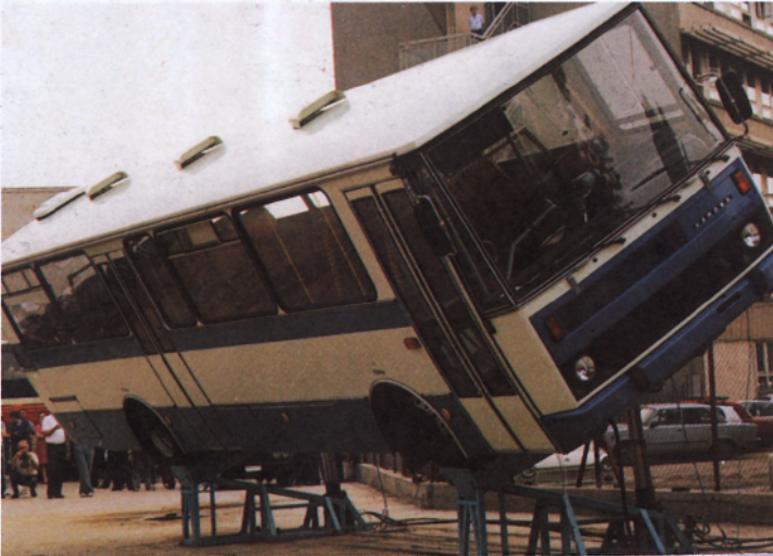
Fig. 4. General arrangement of full-scale test according to ECE R66. A computer controlled hydraulic system with multistep actuators is the basic equipment.
