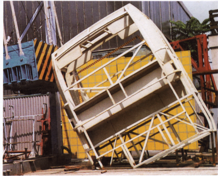
Fig. 7. Pendulum test on a double rear-wall segment of bus IK 396. The results of quasi-static laboratory bending test and the pendulum test indicate big differences on the same segment.
