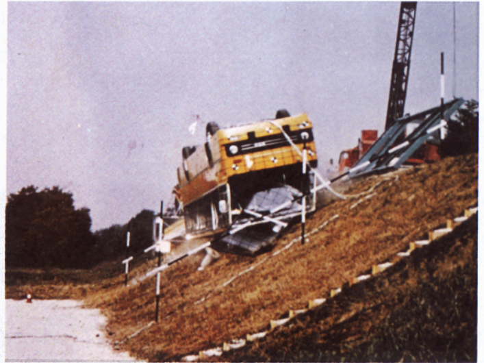
Fig. 3. This 1983's rollover test of Ikarus 255 bus demonstrated the applicability and repeatability of this kind of dynamic test method.
