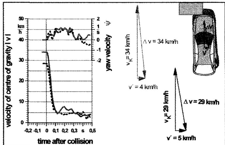
**Figure 7.** Longitudinal decelerations measured on the floor of the passenger compartment and corresponding velocities in the two tests with 29 and 34 km/h collision speed
