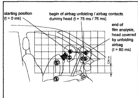
**Figure 12. Movement of the unbelted front passenger dummy in test SH 97.04 (34 km/h, Opel Corsa, Air bags triggered)**
