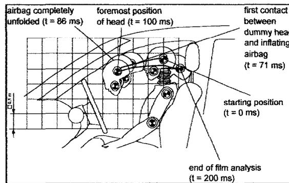
**Figure 14. Movement of the belted driver dummy in test SH 97.04 (34 km/h, Opel Corsa, Air bags triggered)**
