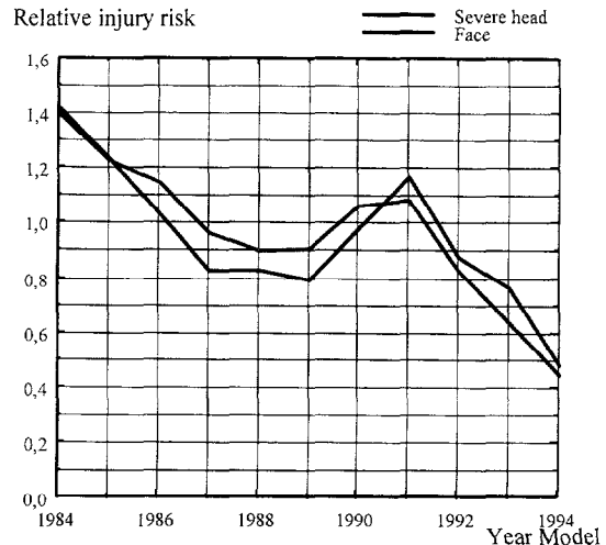
Figure 3. The relative risk of severe skull/brain injuries and facial in car to car collisions with cars of different year model. Facial injuries = 390, skull/brain injuries = 347.
