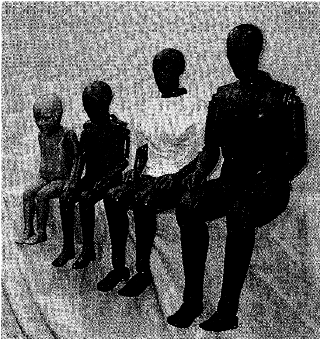
Figure 1. Photograph of the Hybrid III Dummy Family: (left to right) three-year-old, six-year-old small female and mid-size male.
