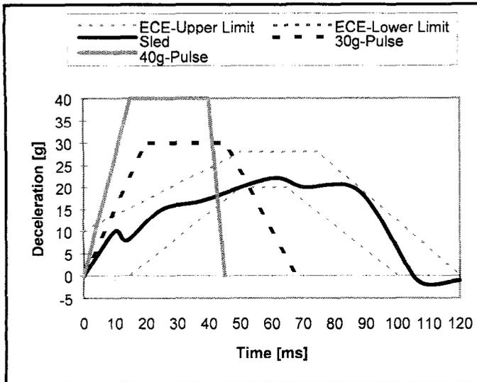
Figure 4. Variation of sled pulses ( $v=50\text{km/h}$ )
