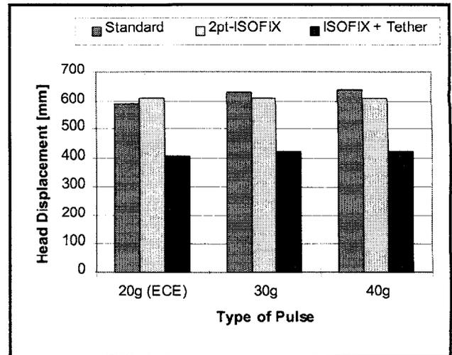
Figure 10. Head displacement
