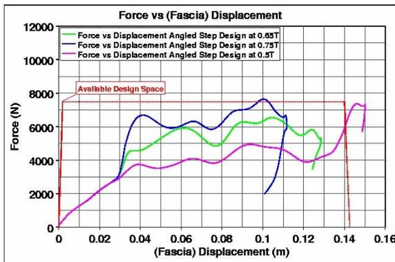
**Figure 9. Impactor force versus stroke results for final 3 step safety plate at variable thickness (7).**
