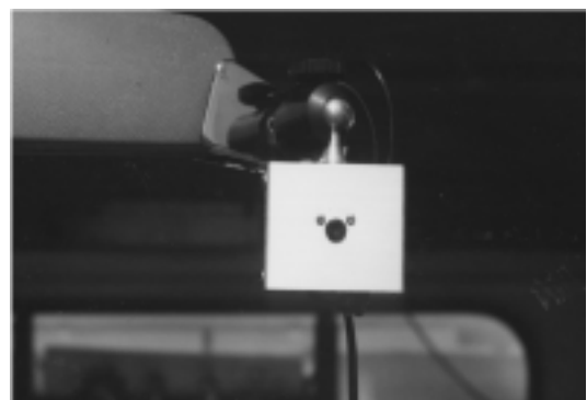
Photo 2. Event Eye Camera Device consists of time lag controller and VTR. The camera was installed in back miller of truck.
