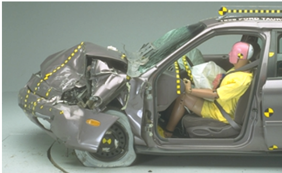
Figure 6d. Crush caused by Lowered ML320
