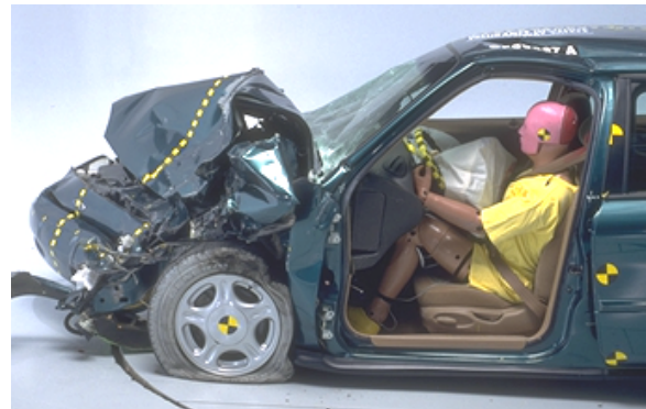
Figure 6b. Crush caused by Normal ML320
