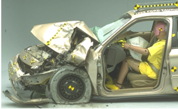
Figure 6c. Crush caused by Raised Rodeo
