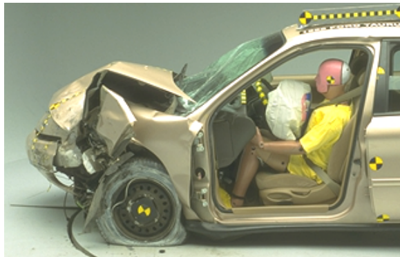
Figure 6a. Crush caused by Normal Rodeo
