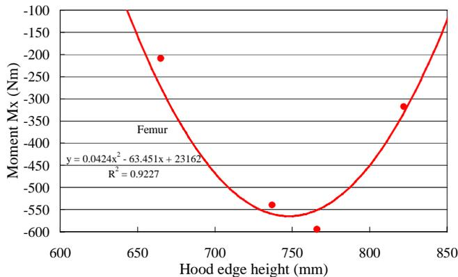
**Figure 11** Hood Edge Height and Femur Bending Moment
