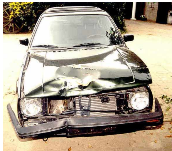
Figure 21. Damage to the Golf
