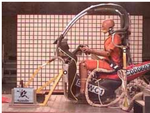
Figure 9. Sled test set-up
